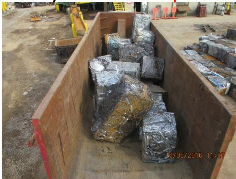
Unevenly loaded trailer – Tip over Risk
